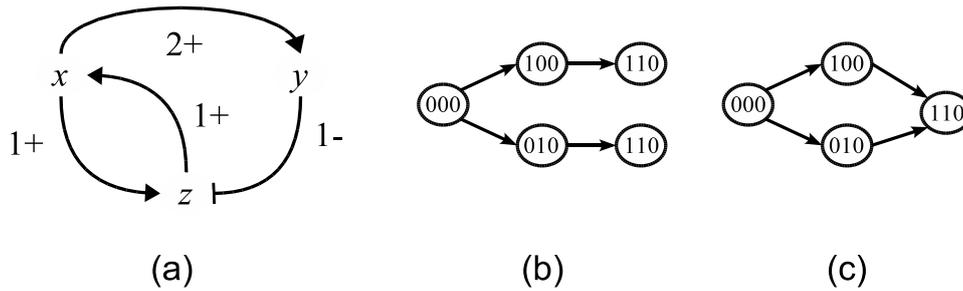
**Figure 4:** Illustration of the reduction of the symbolic execution. (a) is the interaction graph, (b) a part of the symbolic execution, (c) the same reduced symbolic execution.
